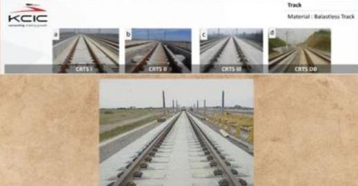
The images show four types of ballastless tracks: CRTS I, CRTS II, CRTS III, and CRTS OD. Each type is shown from a perspective view of the track bed.
