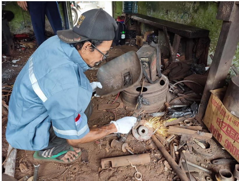
Gambar 2. Proses pemotongan material stainless steel
