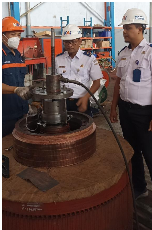
Gambar 13 Proses pelepasan Inner Race Bearing
