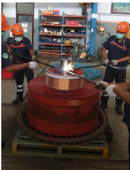
Gambar 1 Proses Pelepasan Inner Race Bearing
