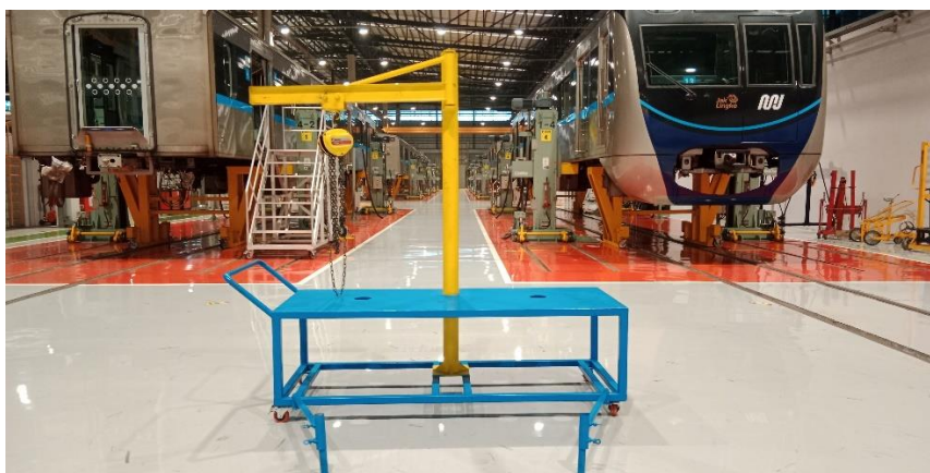
Gambar 9. Alat crane trolley jig air spring
