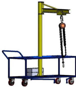
Gambar 3. Desain alat bantu crane trolley jig air spring 3D
