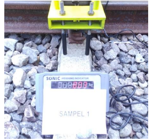
Gambar 6. Proses Pengukuran Kuat Jepit Penambat
